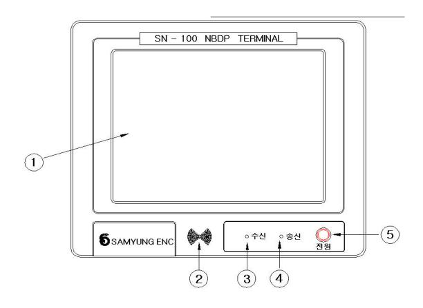
FRONT PANEL (LCD): CHANNEL, TX/RX FREQUENCY, RF.GAIN, CLARIFY, ATT
