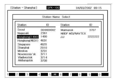
c) After selecting the other station you want to communicate, press [ENT]. Then selected frequency of the other station is printed.
