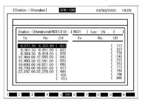
c) Revert the channel you want to communicate using [ ],[ ] key. And then press [ENT] key.
