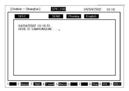
f) As long as connecting with the other station, a curser will be displayed on the left-up side of the screen.
